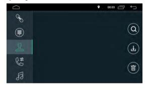
The machine supports syncing of contacts from mobile phone to the machine. Once bluetooth is connected, touch "to download the contacts. Once download is completed, name of the contact will be synced and shown on the display screen during phone call. For
