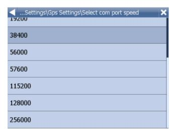
Most GPS receivers work on baud rate of 4800 (but not all). The exact speed should be available in the manufacturers documentation.
