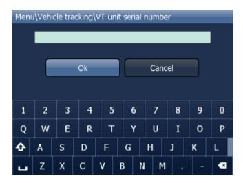
You are now asked to enter the serial number of the VTU008 / VTU009 tracking unit. This number is printed on the underside of the tracking unit.
